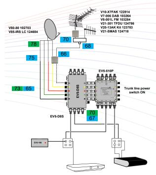
EV5-510P switch "ON" enables the trunk lines to be powered via the receiver or separate power injector / power supply. This ensures that the LNB, Terrestrial and masthead amplifiers to be powered.
