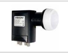
Quattro LNB for IRS systems with four fixed polarity VL, HL, VH, HH. outputs, intended for use with the Vision Sky Q dSCR products or standard IRS switches. This is a very low noise, low gain LNB for maximum quality reception. This LNB is very low current too, making it the ideal choice no landlord supply systems.
