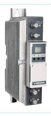
The V90-440 is the professional's solution to large networks and or difficult reception, interference issues, large reception level changes of TV signals The unit enables you to:- Select and level each MUX with AGC; Filter individual MUX / adjacent channels thanks to SAW technology filters; Move MUX's if you wish to re-plan your distribution channels. Each unit is capable of dealing with 4 MUX's simply add units to increase channel capacity. Requires V90-PSU V40-123 / 124548
