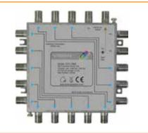
The EV5-1888 IRS Subscriber Power Hub is designed to be used in conjunction with the EV5-1801 Subscriber power injector when there is no landlords mains power supply available. The Subscriber Power Hub provides a means of extracting 18V DC from the SKY Q (SAT 2) feed from the apartment and allowing the dSCR and Legacy switches terrestrial circuits and LNB to be powered.
