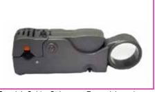
Coaxial Cable Stripper - For quick and easy stripping of WF100 etc coaxial cables. Adjustable double blades strip the centre conductor insulation and remove the outer sheath simultaneously. Guide is printed on the top of the device. Hex key is included for easy blade adjustment. Stripping capacity approximately 4-12mm
