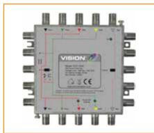
The EV5-1855 IRS Trunk Power Hub is designed to used as power injector where the system requires additional current to supply additional switches in the system. The Trunk Power Hub provides a means of injecting 18V DC at 4 Amps in two directions on V and H lines with DC isolation to prevent the two power supplies conflicting with each other. Full details available online.
