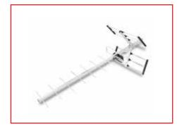
The Y15FAK is a high quality Yagi aerial that has been built for simple, quick installations using a "notools" construction with wing-nuts for the reflector brackets and mast-clamp. The Y15FAK utilises rugged 5mm diameter wire director elements for strength yet low wind loading. These elements are securely staked into the 14mm boom avoiding the use of rivets or screws which can loosen.
