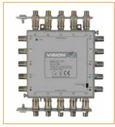
The EV5-110A IRS terrestrial amplifier is designed to be co-located with dSCR and Legacy switches so that extra terrestrial points can be provided in the apartment. This can negate the use of distribution amplifiers in the apartment. With minimal insertion loss up to a total of four switches / amplifiers can be cascaded together.
