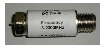
The V17-018 is a coaxial DC block for preventing up to 30V passing along a coaxial cable. These DC blocks are ideal in commercial, IRS or domestic installations where power in one section of a system needs to be separated from another part of a system to avoid overload or backward powering. The DC block is also useful in domestic installations to ensure no DC voltage is short circuited in other equipment such as an aerial dipole or TV tuner.
