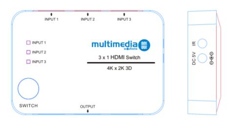
HDMI switches can provide seamless fast switching between HD sources such as satellite receivers, DVD players and other HDMI sources with a remote control or manual switch button. MM20-310A supports 3D TV and HDTV formats up to 4K2K.
