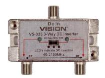
V5-033 is a switchable dual direction DC inserter ideal for remote powering of EV5 systems anywhere in the trunk cable. The DC can be diverted up, down or in both directions in a network. LED indicators confirm the direction of DC powering. V5-033 is fully screened for high RF performance and interference immunity. This model is ideal for remote powering where mains voltage is not available for a headend power supply / amplifier and can also be used to tap off DC voltages to other DC devices.
