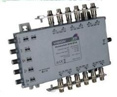
small, medium and large cascaded systems where up to 40 multiswitches can be powered from single V5-034 power source. All multiswitches have stepped gain at each bank of four (eight on 24 & 32) outputs to balance subscriber signal levels and allow long (up to 120m) and short subscriber cables to be connected to the same multiswitch.
