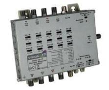
EV5-100T with built-in power supply can be used to power line powered systems including the LNB at up to 2A. EV5-101T can be line powered via its input or output connectors or with a remote power supply (V5-034 recommended). Both models have LED indicators for power on both 14V (V) and 18V (H) line. EV5-100T has additional red/green LEDs for overload or short-circuit identification.
