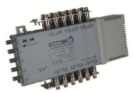
powered multiswitches can be used to power up to six line powered multiswitches and an LNB. EV5-xxxM will power a Quattro LNB via the horizontal inputs at up to 650mA max. Power is provided from the built-in switch-mode power supply.
